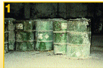
1 Obsolete stocks discovered in a warehouse where they had been abandoned years before. Some barrels were leaking as a result of corrosion.
