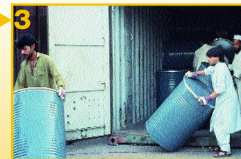
3 Offloading the empty UN barrels which are approved for safe transport under the International Maritime Dangerous Code.
